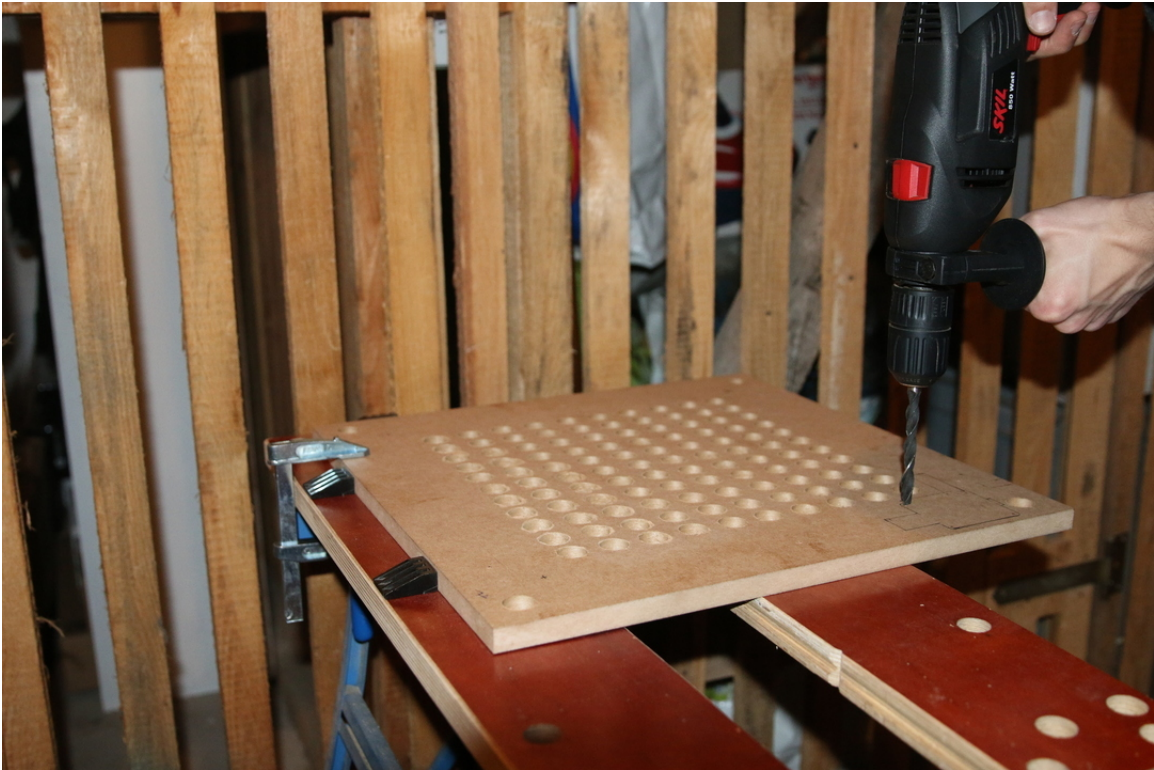
Fig. 1: According to the stencil layout, for each LED a hole needs to be prepared. The total number of 114 holes makes this pretty tedious.
