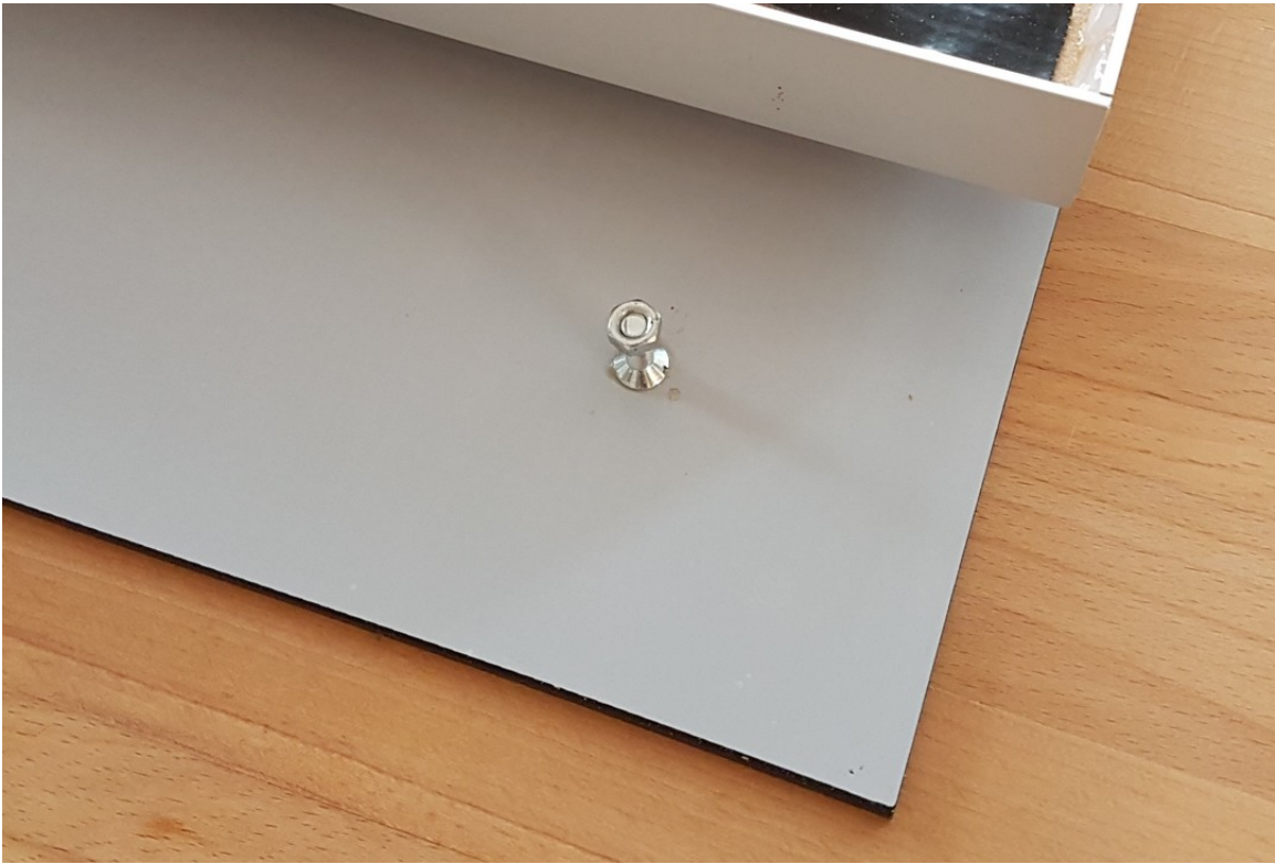
Fig. 11: Allows to fix the stancil with screw-nuts to the sceleton.
