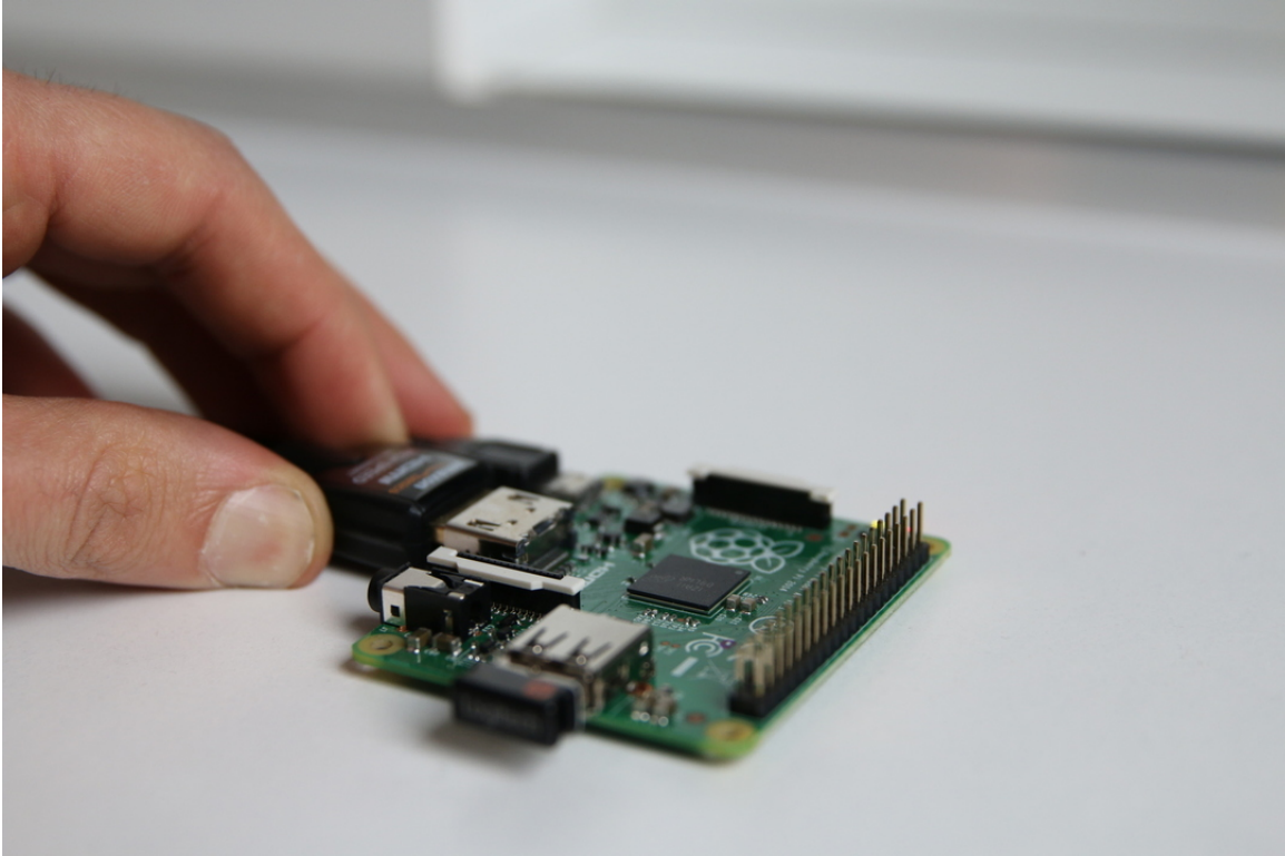
Fig. 5: Before you mount your raspberry inside the clock, install the latest Raspbian, connect it to your local wifi and ensure that you can ssh to it.
