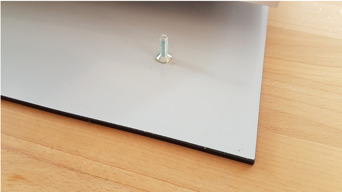
Fig. 10: Fixation of 4 screws within the 4 corners of the stencil using two-component adhesive.
